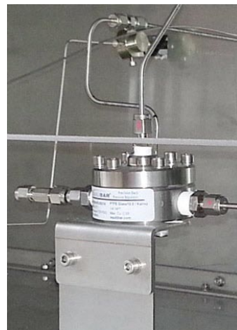
Figure 5: The image above shows Equilibar's LF Research Series back pressure regulators installed in an Integrated Lab Solutions system.
