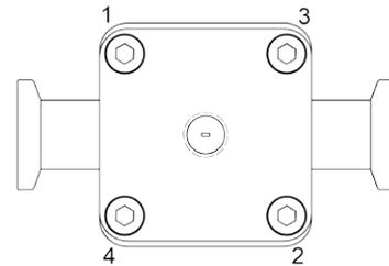
Figure B: Sample Torque Pattern
