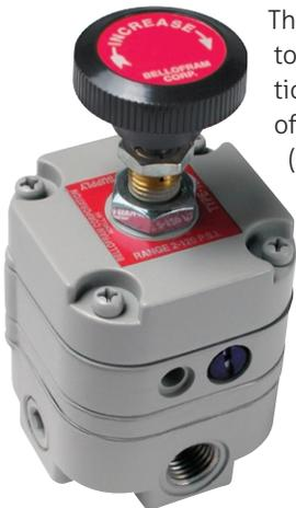
There are numerous precision air regulators targeted at instrumentation applications in the range of 1/8" or 1/4". Several of these can control pressures below 1 psig (69mbar), though no commonly available solutions are precise in the ultra low range. These regulators typically are self-relieving, meaning that they can vent downstream air when the set-point is lowered or if the downstream
