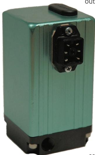
These EPRs typically require a DC power supply and a set-point signal. Analog controllers typically accept either current (4-20 mA) or voltage (typically 0-10 or 0-5 VDC) input. Models with digital circuits can accept serial communications (such as RS-232 or Ethernet) in addition to the common analog standards. Most models also offer a feedback signal reporting on the pressure sensor value.
