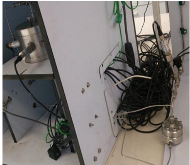
Figure 3: High-pressure Experimental Rig for Supercritical CO 2 and Water System (Equilibar Back Pressure Regulator at the bottom right)
