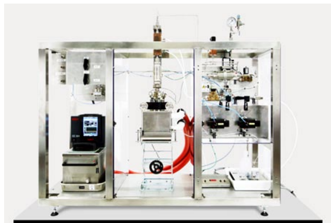
Figure 2: Hydrofluoric Acid research system built by Integrated Lab Solutions with the installation of the Equilibar® regulator.
