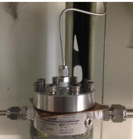
**FIGURE 4.** Left Picture: The BPR as installed in the Duke SCWO unit. High pressure fluid enters from the left and leaves at ambient pressure on the right. The smaller process line entering from the top is the charged pressure applying force to the floating diaphragm. Right Picture: The BPR with the top and diaphragm removed.
