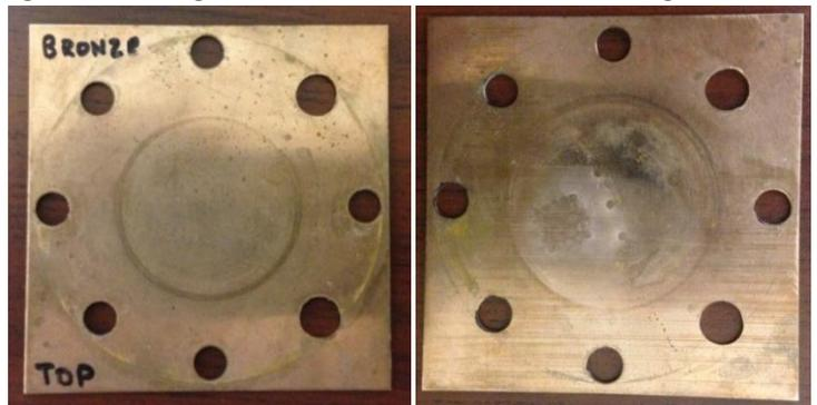
**Figure 5f.** Top and bottom view of a titanium diaphragm used in the Duke SCWO unit. Diaphragm was made in-house, and has shown no signs of wear after over 12 hours of operation.
