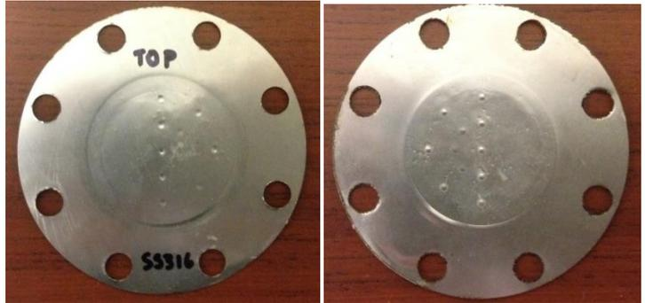
**Figure 5d.** Top and bottom view of a stainless steel diaphragm, thicker than the standard SS8, used in the Duke SCWO unit. This thicker stainless steel diaphragm was only subjected to 2 hours of pressure testing, and showed some signs of fatigue.
