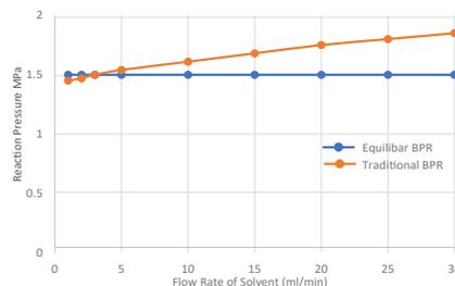
Figure 2: Graph of reactor pressure control at various flow rates with an Equilibar back pressure regulator versus a traditional unit
