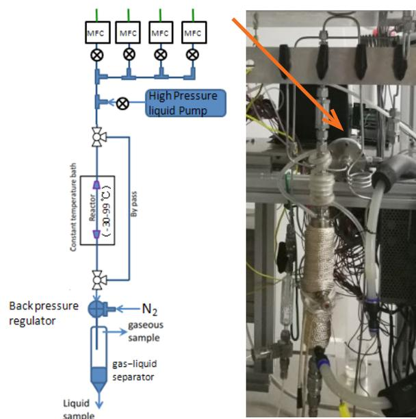
Figure 3: Direct synthesis reactor schematic and photo with an Equilibar LF1 back pressure regulator indicated by an arrow.
