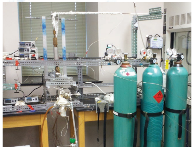
Lab set-up showing Fischer Tropsch Synthesis reactor (foreground, insulated) with flow control instrumentation
